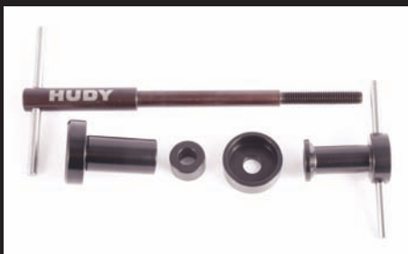
Above: Front bearing remover and installer for both
