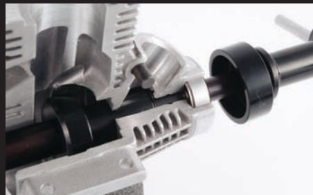
Above: Ready to pull out the front bearing
