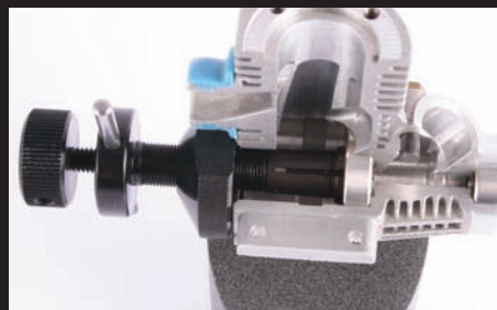
Above: Ready to remove the rear bearing – just turn the knob
