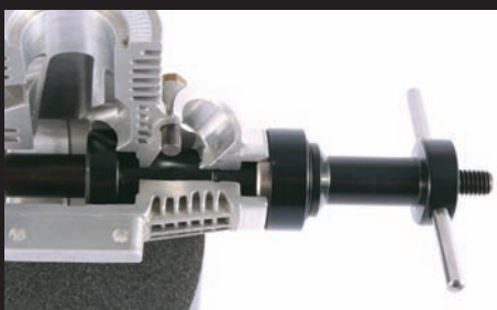
Above: Front bearing out in stages
