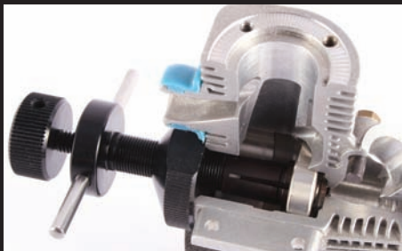
Above: Steps of bearing coming out
