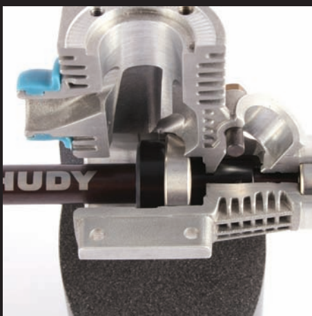
Above: Both front and rear bearings going in together
